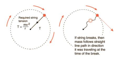
The string must provide the necessary <u>centripetal force</u> to move the ball in a circle. If the string breaks, the ball will move off in a **straight line with constant speed**.
